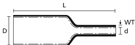
Heat Shrinkable Tubing 4:1 with adhesive
