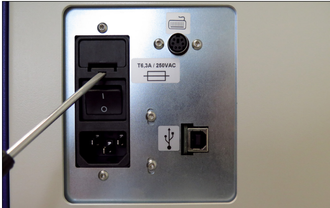
Replacing the power input fuse.
