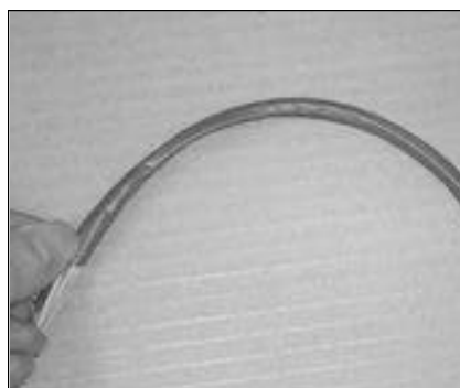
17. Apply PVC tape to the fibre units at position 'C'.
