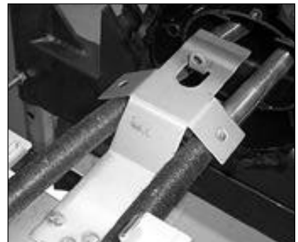
24. Place organiser in between the cables and fit to the base, secure using the screws.
