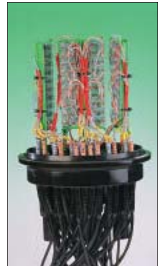
CDJ with Channell terminal blocks
