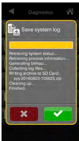
Figure 26 System log saving
