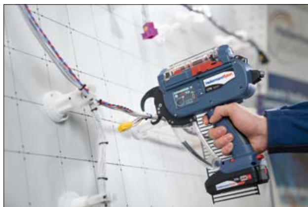
Battery-operated Autotool CPK hybrid applying cable ties from bandolier.
