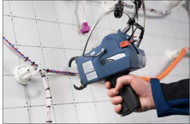
Autotool ATS flex on the harness board (also shown: Overhead suspension ATS).
