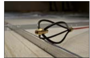
The whisk allows the rod to glide over obstructions easily.
