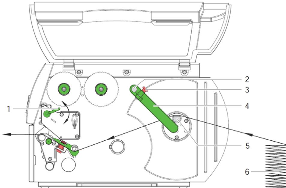
**Figure 8** Loading fanfold labels
