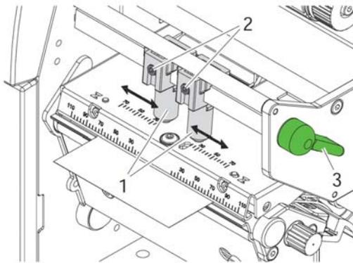
The print head is pushed on via two plungers (1). In the basic setting the plungers are set in the middle of the print head retainer. This setting can be used for the most applications.
